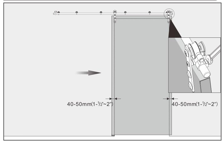
As shown in the figure, adjust to the appropriate position with a wrench to tighten the screws
