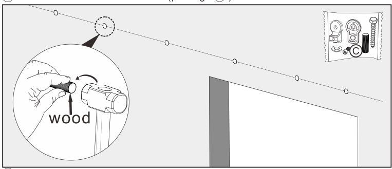
(4) Marking and drilling holes in wood anchors
