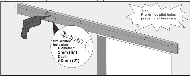
7 Package Cpart mounting location (no wood anchor required)
