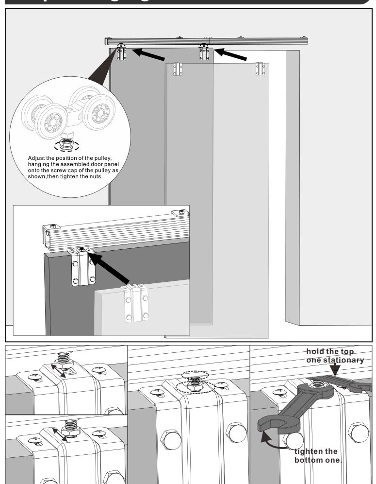
1) Fine-tuning the front and rear 2) Tighten the screws in the positions of the door panels picture
