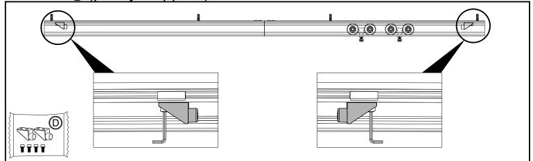
Step 2: Install the track ("Plasterboard Wall" and "Wood Frame Wall" installation process in P7-P9; "Concrete Wall" please check P10~P11)
