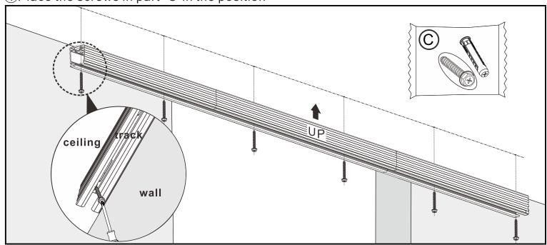
②Adjust the track position until the top edge of the track is tight against the ceiling, then tighten the screws.
