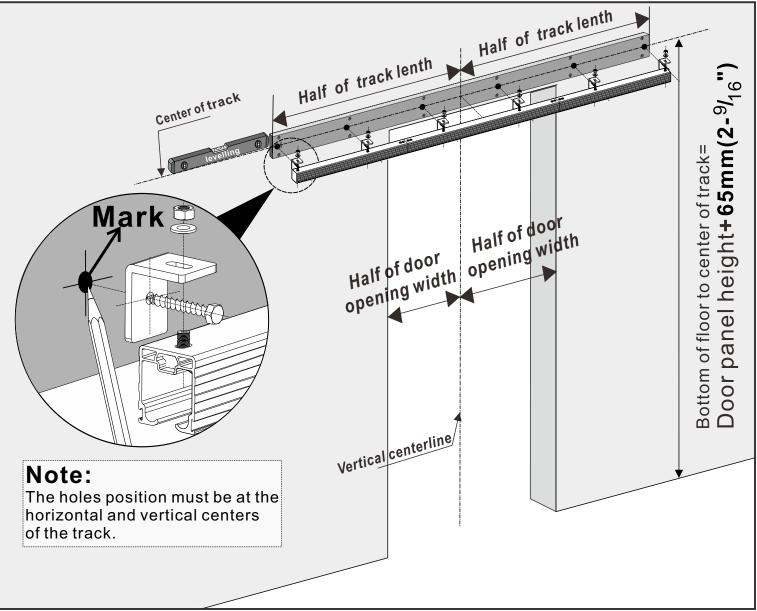
(5) Refer to the dimensions in the attached table and proofread the dimensions again with a tape measure
