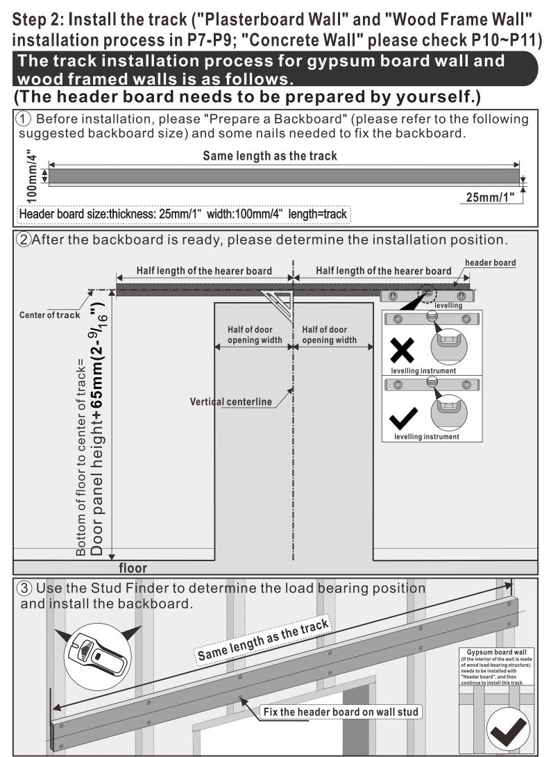
The track installation process for gypsum board wall and wood framed walls is as follows.
