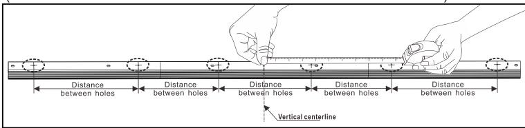
4 Drill holes in the track according to the marked positions
