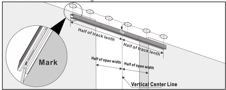
②Drill 50mm(2") deep holes in the roof with a 11mm( $^{7}$ / $_{6}$ ") diameter drill bit
