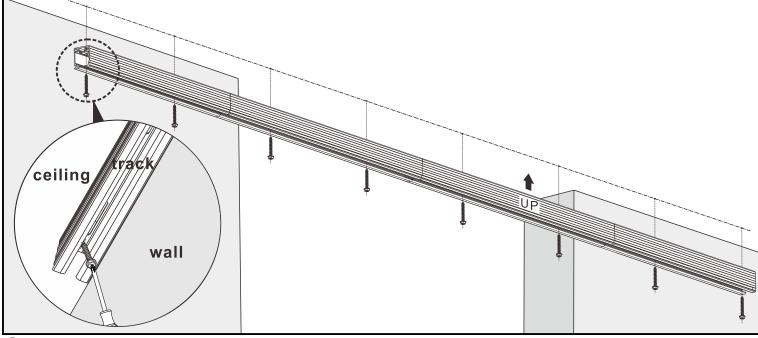
2 Adjust the track position until the top edge of the track is tight against the ceiling, then tighten the screws.
