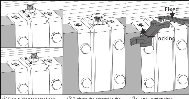
1 Fine-tuning the front and rear positions of the door panels.
