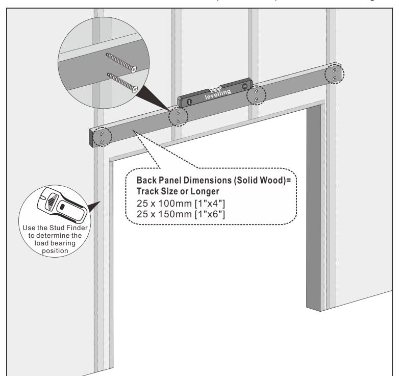
Note: Please prepare the back panel and the components for installing the back panel yourself.
