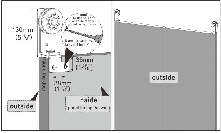
②Install the pivot sleeve at the bottom of the door.
