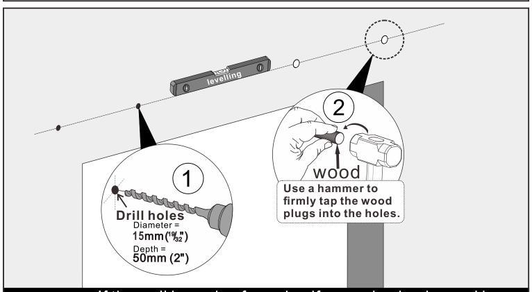
Note: If the wall is made of wood or if a wooden back panel has already been installed, please skip this step.
