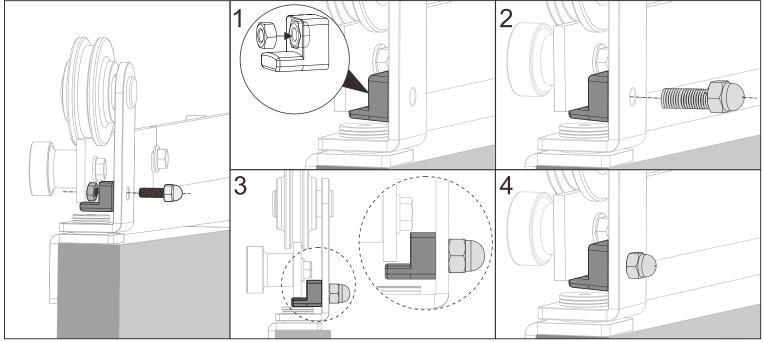
Install the U-shaped fixing fittings.
