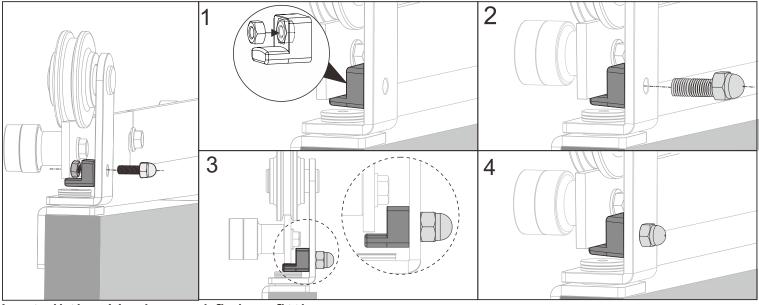
Install the U-shaped fixing fittings.
