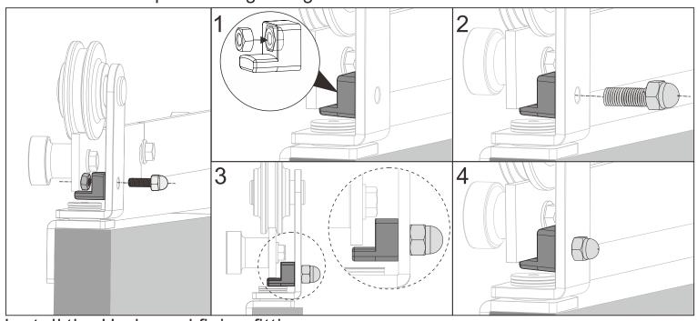
Install the U-shaped fixing fittings.
