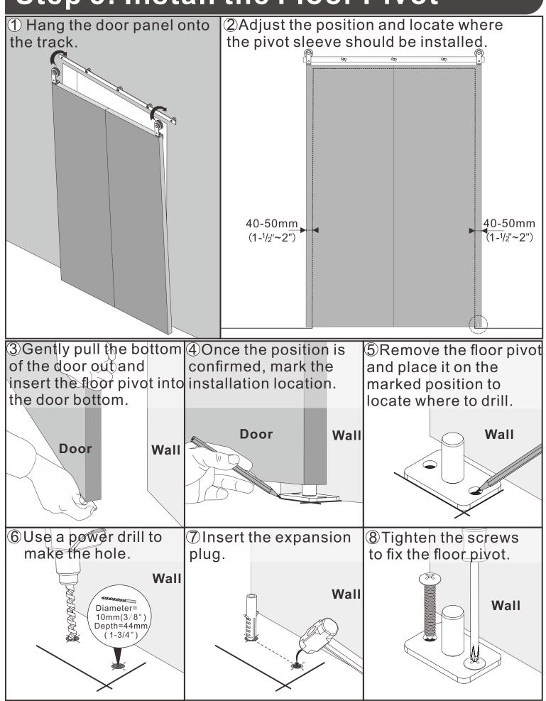
If your floor is made of wood and the depth is greater than 40 mm (1-9/16"), please use a 3 mm (1/8") drill bit to pre-drill a guide hole, and there is no need to install the expansion plug.
