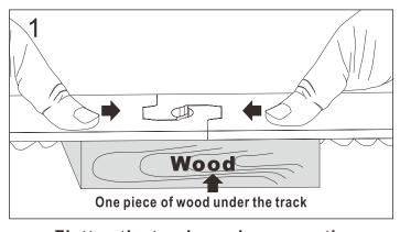
Flatten the tracks and squeeze the two tracks towards the middle
