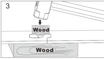
Place a piece of wood on top of use a hammer to secure it into the track
