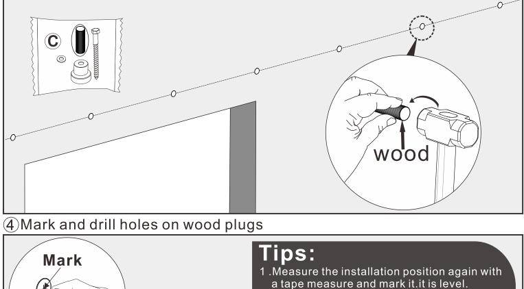
Drill deep 50mm(2") holes with 3mm(<sup>1</sup>/<sub>8</sub>") power drill.
