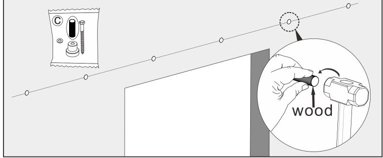
④Refer to the dimensions in the attached table and proofread the dimensions again with a tape measure(Mark the location of the punch on the wood nails.)
