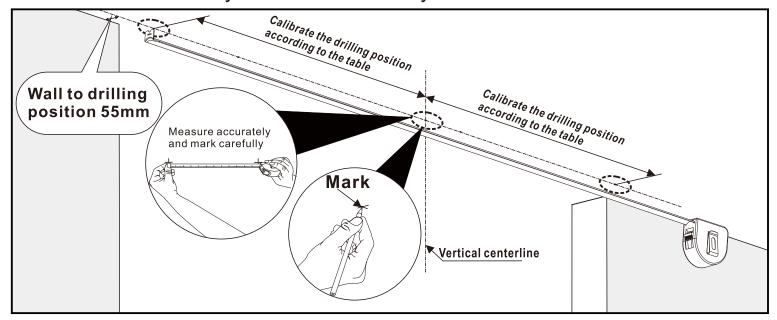
4Drill 50mm(2") deep holes in the roof with a 11mm( $^{7}$ /<sub>16</sub>") diameter drill bit
