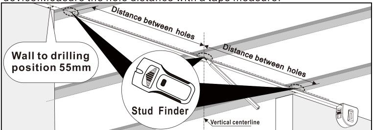
3 Mark the hole spacing on the track according to the measured distance (if the marked position is not a pre-drilled position, it is necessary to re-drill the holes in the track) (along the contribute of the track)
