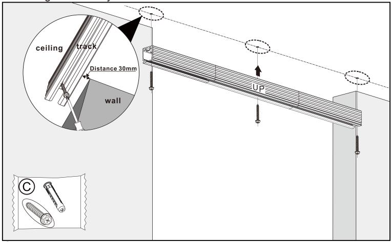
②Adjust the track position until the top edge of the track is tight against the ceiling, then tighten the screws.
