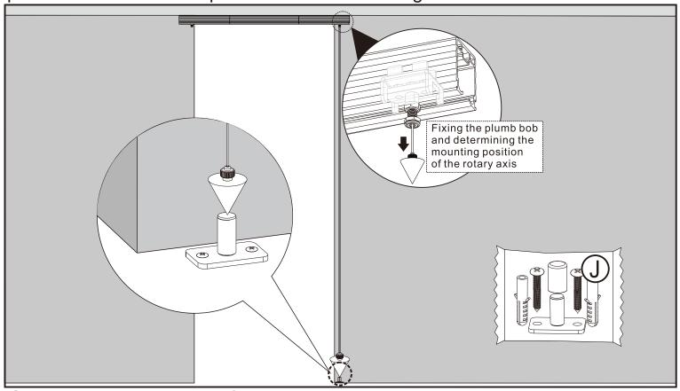
2 Prepare the package Ucomponents for installing the pivot axis.
