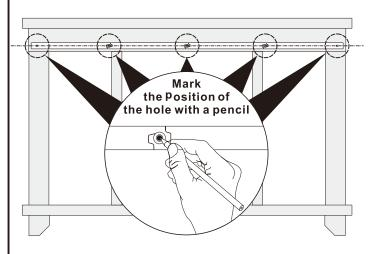
4 Determine the location of the drilled holes again with a tap measure according to the attached table for the different sizes of track.
