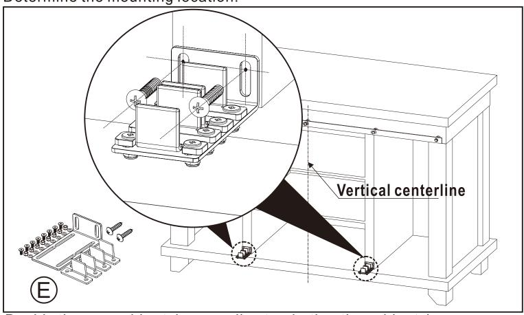
Decide the assembly style according to whether the cabinet door is slotted or not (do not tighten the screws first).
