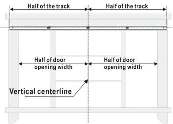
3 Place the splicd track on the position and mark the location of the holes to be drilled.
