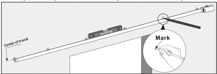
$\bigcirc$  Drill deep 50mm(2") holes with 3mm(  $\frac{1}{8}$  ") power drill
